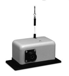
The PT420 is available with full-scale measurement ranges from 2 to 100 inches, providing a 0/4-20 mA feedback signal that is linearly proportional to the position of a traveling stainless-steel extension cable. Use the PT420 to provide position feedback on hydraulic cylinders in factories and utilities, gate position in fresh or wastewater distribution systems, or valve opening in process-related applications.
