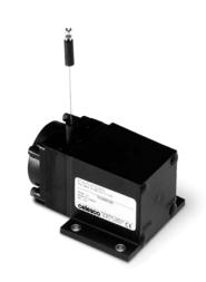
The PT1DN communicates to your PLC over DeviceNET° and provides a precision position feedback signal for full-scale measurement ranges from 2 to 50 inches. Because the PT1DN uses a potentiometer as it's sensing element, the position signal is "absolute" and does not have to be reset to a "home" position upon startup.
