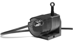
The MT3A is the solution for high-acceleration test applications in potentially wet environments. Just like the MT2A, the MT3A comes in 4 different full-stroke ranges, has a high-tension heavy-duty measuring cable designed for the demands of flight and automotive crash tests and comes with an easy to use 2-axis 360° rotation mounting bracket for installation in hard to fit areas.
